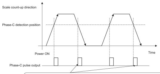
The phase-C pulse is also output when the detection head of the encoder passes this point in reverse, because the SERVOPACK has recorded the position where the phase-C pulse was originally output when first passing the position in the forward direction.
