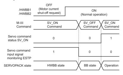
Note: Even if the servomotor power is turned OFF by turning OFF the main circuit power, the HWBB status is retained until a servo OFF command is received.
