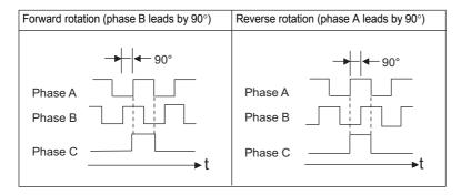
Note: The pulse width for phase C (origin pulse) changes according to the setting of the encoder output pulses (Pn212) and becomes the same as that for phase A.
