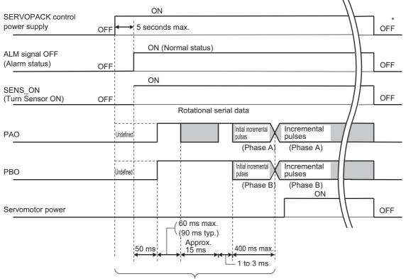
The servomotor will not be turned ON even if the SV\_ON command is received during this interval.
