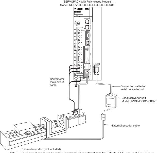
Note 1. The figure above shows a connection example of an external encoder. Refer to 1.5 Examples of Servo System Configurations for details on the power supply and peripheral devices.
