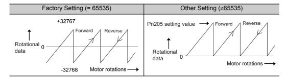
Note: The standard specification of the direct drive motor include an absolute encoder that shows values for a single rotation, so the multiturn data (rotational serial data) for the encoder is always 0. The absolute value of the load side can be created with the motor shaft angle only even when constructing an absolute position detecting system because the servomotor and the load can be directly connected.
