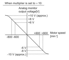
Note: Linear effective range: within  $\pm$  8 V Output resolution: 16-bit
