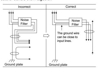
Connect the noise filter ground wire directly to the ground plate. Do not connect the noise filter ground wire to other ground wires.
