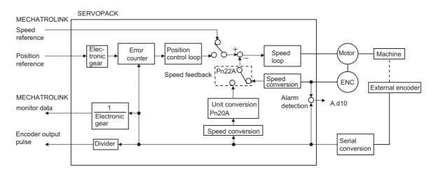
Use Pn22A.3 to select the speed feedback method during fully-closed loop control: Normally, set Pn22A.3 to 0 (Uses motor encoder speed.). Set Pn22A.3 to 1 (Uses external encoder speed.) when connecting a direct drive motor and high-resolution external encoder.
