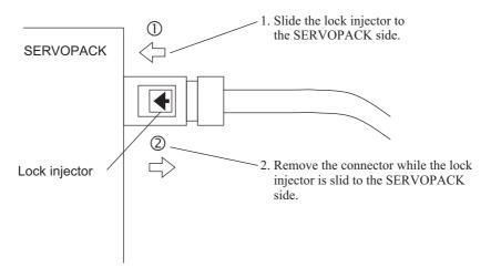
Note: The MECHATROLINK-III communications cable connector may be damaged if it is removed without being unlocking.
