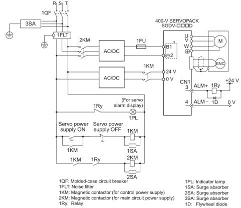
Terminal names differ depending on model of SERVOPACK. Refer to (2) DC Power Supply Input Terminals for the Main and Control Circuits.
