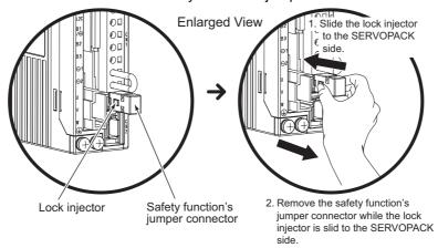
Note: The safety function's jumper connector may be damaged if removed while the lock is still on.
