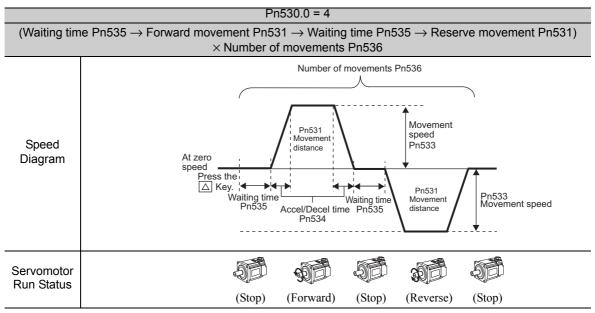
Note: When Pn536 (number of times of program JOG movement) is set to 0, infinite time operation is enabled. To stop infinite time operation, press the JOG/SVON Key to turn OFF the servomotor power.
