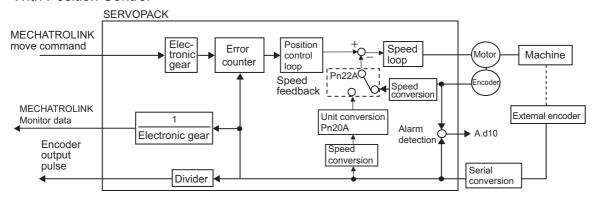
Note: Either an incremental or an absolute encoder can be used. When the absolute encoder is used, set 1 to Pn002.2 (use the absolute encoder as an incremental encoder).
