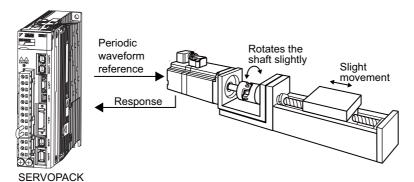
In addition to this function, online vibration monitor (Fn207) can be used to detect machine vibration and automatically make notch filter settings.
