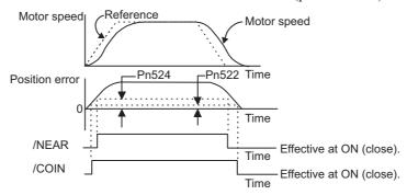
Note: Normally, the value of Pn524 should be larger than that for the positioning completed width (Pn522).
