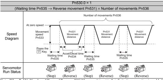
Note: When Pn536 (Number of Times of Program JOG Movement) is set to 0, infinite time operation is enabled. To stop infinite time operation, press the JOG/SVON Key to turn the servomotor power OFF.
