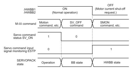
The HWBB function operates while the servomotor power is ON.
