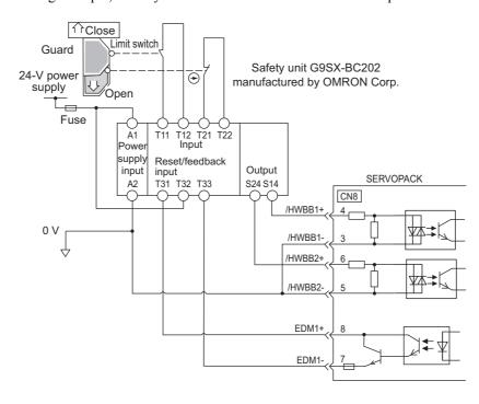
When a guard opens, both of signals, the /HWBB1 and the /HWBB2, turn OFF, and the EDM1 signal turns ON. Since the feedback is ON when the guard closes, the safety unit is reset, and the /HWBB1 and the /HWBB2 signals turn ON, and the operation becomes possible.
