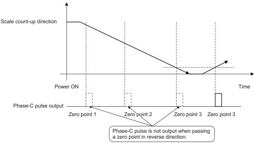
To output the phase-C pulse when a detection point is passed in reverse, set the following parameter to 1.
