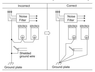
If a noise filter is located inside a control panel, first connect the noise filter ground wire and the ground wires from other devices inside the control panel to the ground plate for the control panel, then ground the plates.
