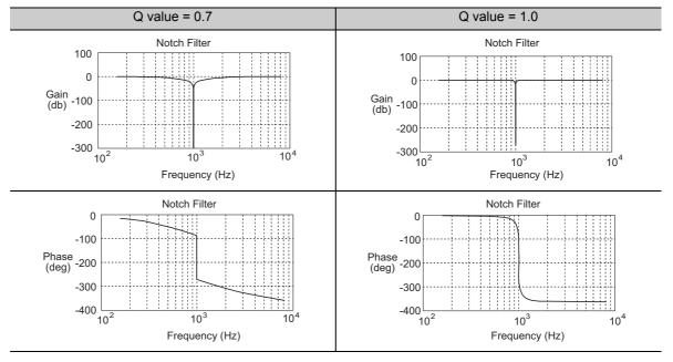
The notch filter can be enabled or disabled with Pn408.
