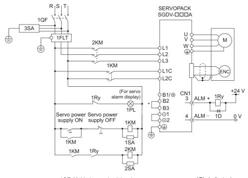
1PL: Indicator lamp 1QF: Molded-case circuit breaker 1SA: Surge absorber 1FLT: Noise filter 1KM: Magnetic contactor (for control power supply) 2SA: Surge absorber
