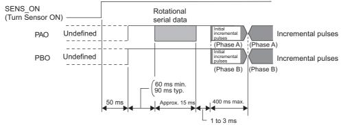
Note: The output pulses are phase-B advanced if the servomotor is turning forward regardless of the setting in Pn000.0. Rotational serial data:
