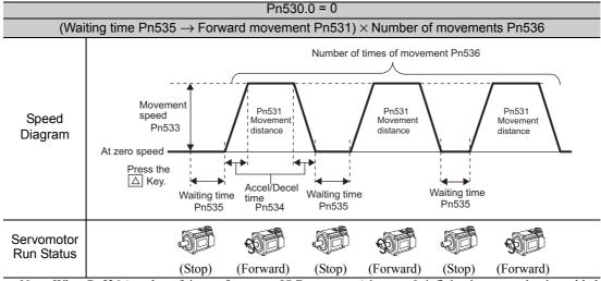
Note: When Pn536 (number of times of program JOG movement) is set to 0, infinite time operation is enabled. To stop infinite time operation, press the JOG/SVON Key to turn OFF the servomotor power.
