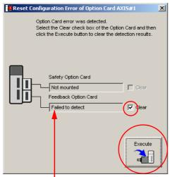
You cannot clear the **Error detected** detection result. Remove the Option Module, or check to see if the Option Module is correctly mounted.
