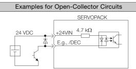
Note: The 24-VDC external power supply capacity must be 50 mA minimum.
