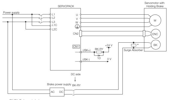
BK-RY: Brake control relay 1D: Flywheel diode
