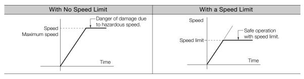
Note: The actual limit of motor speed depends on the load conditions on the Servomotor.
