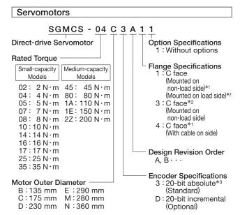
\*1: Only for small-capacity models. \*2: Only for medium-capacity models.
