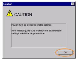
6. Turn the power supply to the SERVOPACK OFF and ON again after the parameter settings have been initialized.
